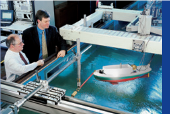
VWT model with Voith Turbo Fin at the Voith in-house marine test laboratory
